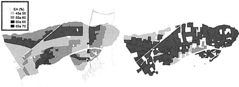
Fig. 1. Map of Application Efficiency (EA, %) for the situations before (left) and after (right) the modernization process.
