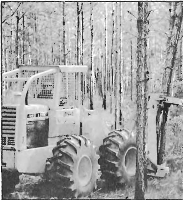
Fig. 13. Cizalla John Deere.
