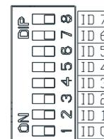
**Example:** If you need to set the address of RTU-485 to 26, switch the DIP switch corresponding to ID4 to "ON", switch corresponding to ID3 to "ON" and switch corresponding to ID1 to "ON".
