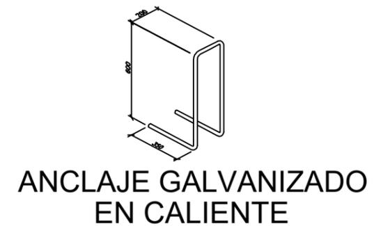
ANCLAJE GALVANIZADO EN CALIENTE
